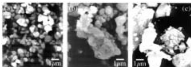
Figure 2. SEM images for \text{Sr}_2\text{CeO}_4 particles obtained by the (a) calcination of the co-precipitated carbonate at 1373 K, (b) solid-state reaction at 1373 K, and (c) solid-state reaction at 1573 K.
